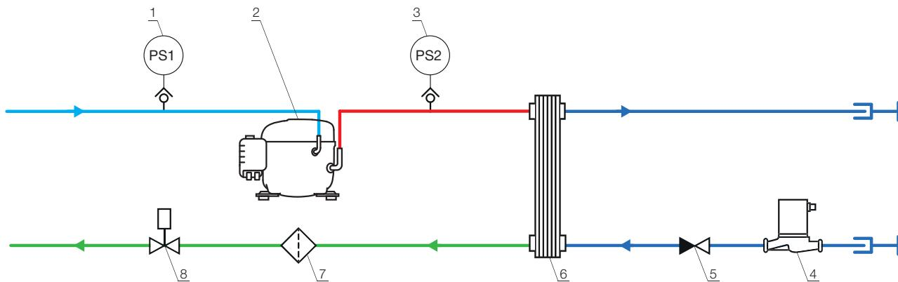
1 - Low pressure relays with fixed settings (mini pressure switch)
